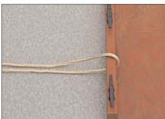
If the line starts under the bull rail on the dock it is easier to feed it back to the boat. Feed it under the bull rail and back over the bull rail to a boat cleat when possible. Your crew can then cast off the mooring lines without leaving the boat or doing the "Leap of Death" to get back on board.
