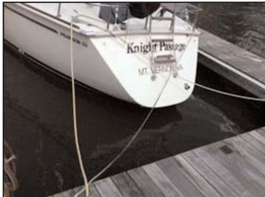
Figure 4 – Stern Lines crossed to cleats on a dock
