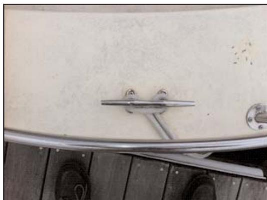
Figure 5 – Dock line secured to a cleat on a boat
