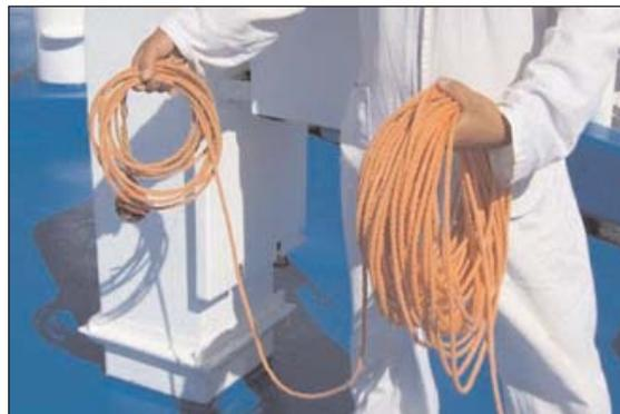
Figure 6 splitting the coil
